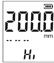
High alarm limit setting.
